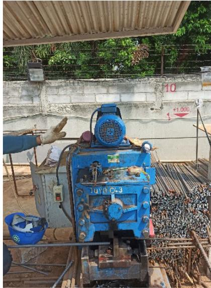
**Gambar 2.3** Bar Cutter Electric
