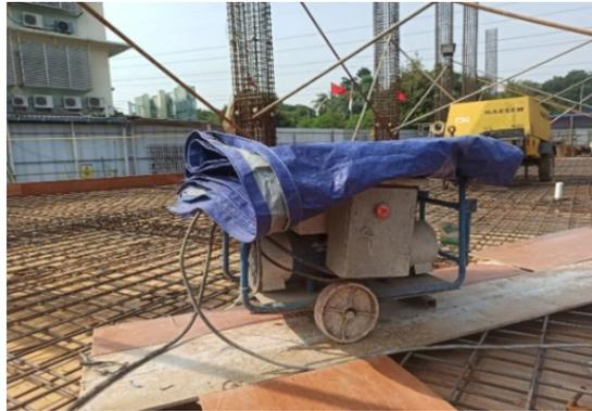
**Gambar 2.4** Concrete Vibrator
