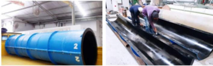
Gambar 1.4. Bekisting Fiberglass
